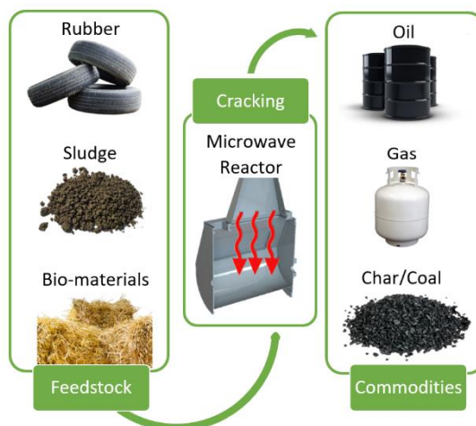
Figure 1 – Basic principle of the OFT process
